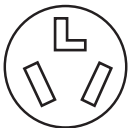
3-wire receptacle (10-30R)
